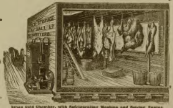
Small cold Chamber, with Refrigerating Machine and Sewing Engine.
